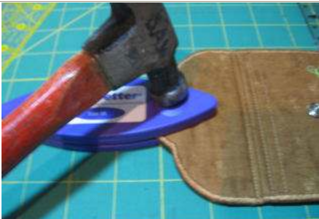
17. Slip the top section of the snap setter tool over the middle tool piece. Hammer the snap parts into place.
