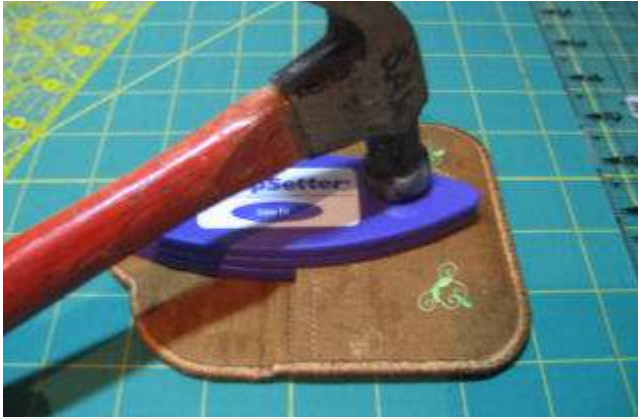
13. Slip the top section of the snap setter tool over the middle piece. Hammer the snap parts into place.
