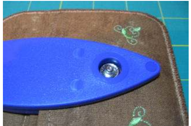
12. Slip the middle section of the snap setter tool over the bottom piece. Place the snap stud inside the hole on the snap setter tool.
