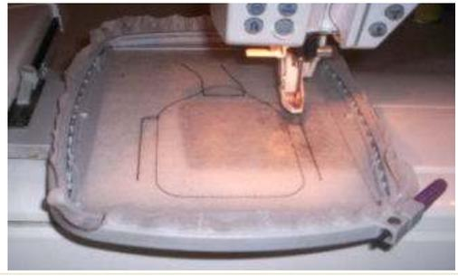
10. Send the cell base design to machine. Hoop vilene in hoop. First outline sewn directly on vilene. (no fabric yet) Also stitches placement lines for tab at top and the pocket.
