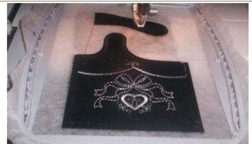
6. The last step stitches the satin edge across the top of the pocket and around the tab.
