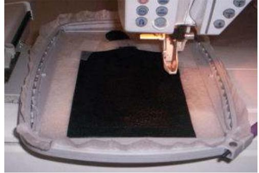
12. The next step tacks the fabric & felt for the base down. Remove hoop, trim fabric/felt from around shape on both sides of hoop. Be careful not to cut into the tab at the top!
