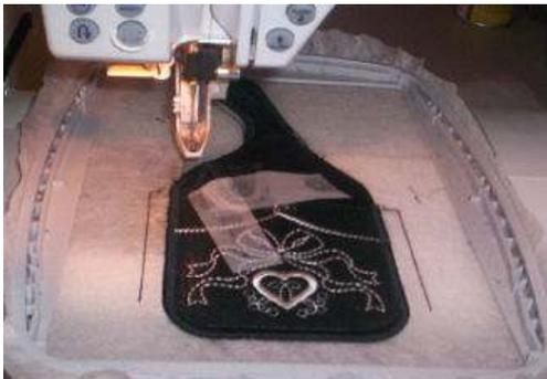
13. The last step in the design stitches the final satin edging around the cell pouch covering the raw edges of the fabric. Keep tab taped down out of the way.
