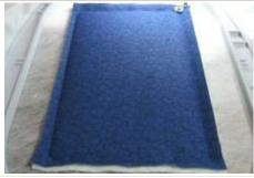
4. Place hoop back on machine. The second color tacks the fabric/batting down on both sides of the hoop & stitches little notches on the ends to aid in pocket placement.
