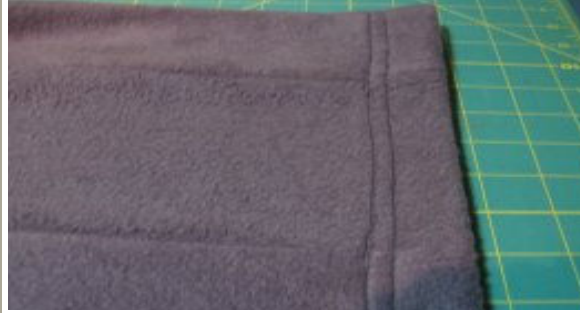
10 - Fold top to 3" line and top stitch 1/4" from cut edge. Stitch another row 3/8" above first row of stitches to create channel for the plastic tubing.
