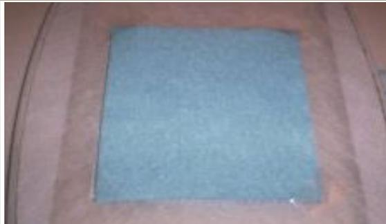
4. Flip hoop over, center felt over outline, tape at corners and put hoop on machine.
