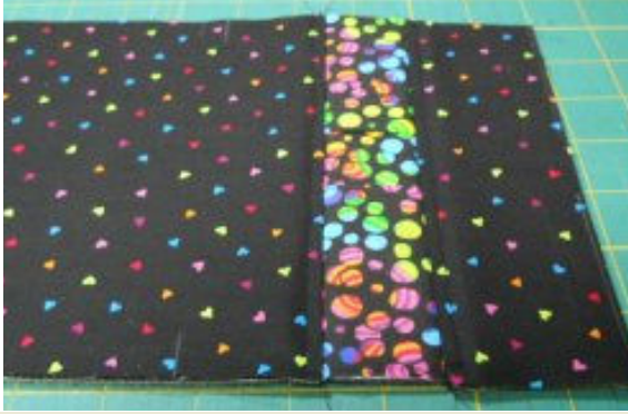
31. Rub glue stick on edge of soft & stable, smooth top & bottom fabrics down, iron to set. Top stitch seams.
