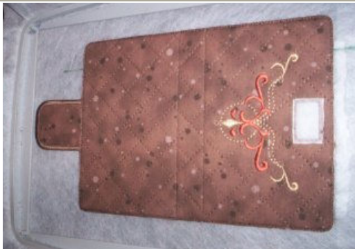
Case 13 - Remove hoop & trim fabric/felt close to outline stitches on both sides of hoop. Take care to avoid cutting into the tab when trimming! Put hoop back on machine.
