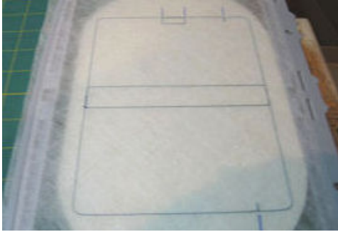
Case 1 - Stitch outline on stabilizer only. Pocket placement notches stitched at top/bottom & narrow rectangle stitched at top center for tab placement. Flip hoop over & extend all notches by marking 1" lines on the stabilizer.
