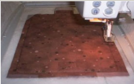
Case 5 - Center fabric over felt/batting. Tape in place, put hoop on machine. Next step tacks fabric/ tab down & stitches small rectangle outline for velcro placement.
