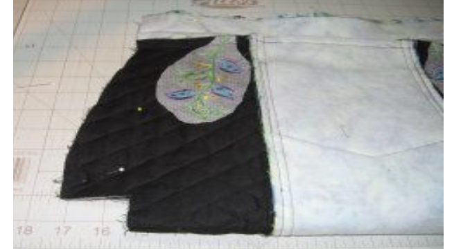
20. Pin purse sides together (top band is opened flat) and stitch sides with 1/2" seam.
