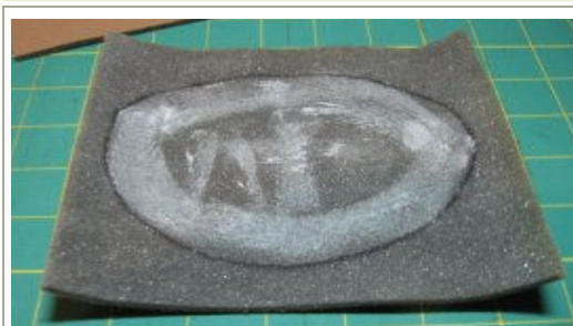
28 - Center smaller template on wrong side of headliner fabric & trace. Spread glue inside outline (Scotch glue stick) & press "shaped" canvas down over the glue.
