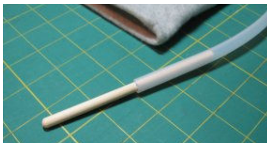
23 - Mark center of dowel and push dowel inside plastic tubing up to the dowel center mark.
