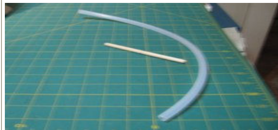
22 - Cut 3/8" OD polyethylene tubing and 1/4" dowel rod to length. Round ends of dowel rod with sand paper.
